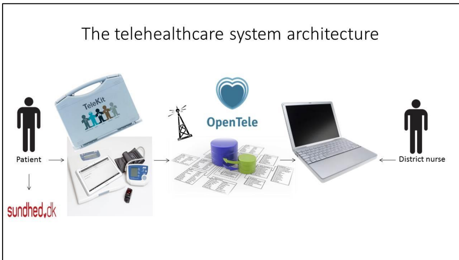
Figure 6: The Telekit system framework. At home, patients were guided through their measurements using a tablet application. Devices used to measure the patients' vital signs were connected to the tablet through Bluetooth. Patients could view their measurements via the tablet or the public health portal ( www.sundhed.dk ). The data were sent by patients to a central server, OpenTele, which stores data and ensures data exchange between relevant entities. District nurses could view the data from the web portal, OpenTele, and contacted the patients if deviations in their measurements occurred.
