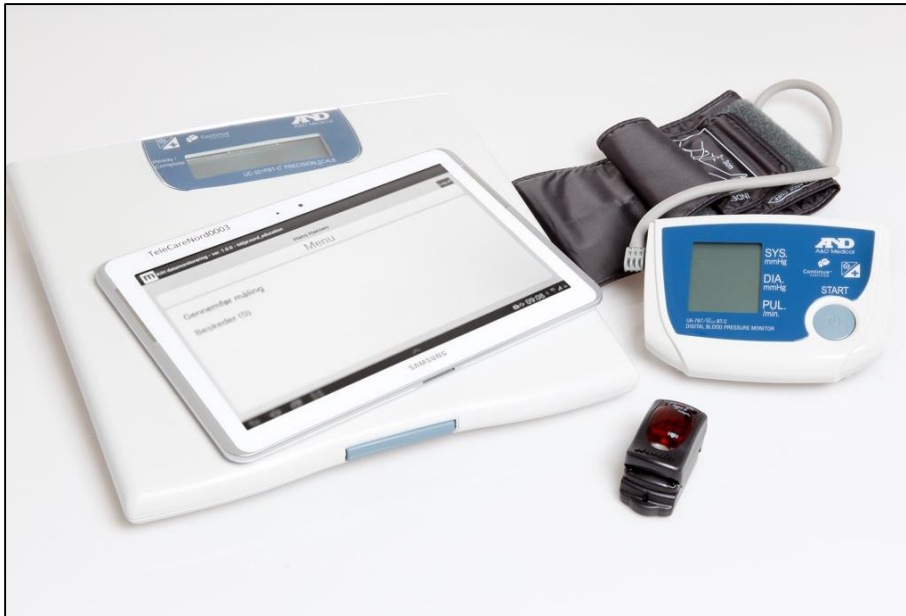
Figure 3: The telehealthcare system, Telekit, consists of a tablet, a blood pressure monitor, a fingertip pulse oximeter, and a weight.
